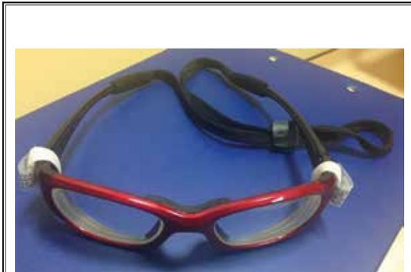
Fig. 2. Position of dosimeters on lead glasses.
