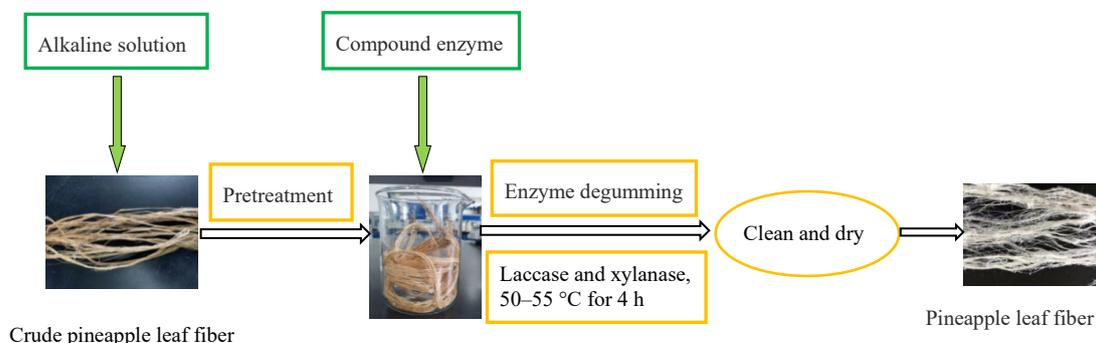
Figure 1: Process flow diagram of PALF degumming
