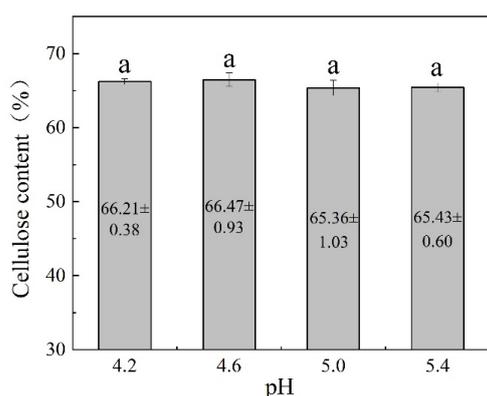
Figure 2: Effect of pH during PALF degumming on cellulose content (different lower case letters indicate significant differences ( $p < 0.05$ ))
