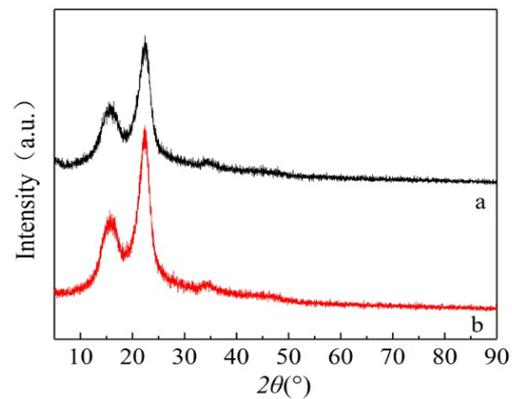
Figure 7: X-ray diffraction patterns of (a) non-degummed and (b) degummed PALF
