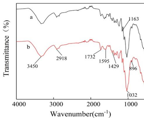
Figure 6: FTIR spectra of (a) raw and (b) degummed PALF (characteristic peak values indicated on the graph)
