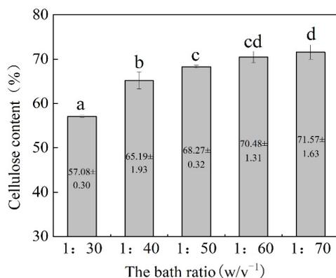
Figure 4: Effect of bath ratio during PALF degumming on the cellulose content (different lower case letters indicate significant differences ( $p < 0.05$ ))
