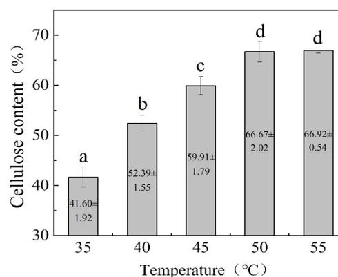
Figure 3: Effect of temperature during PALF degumming on the cellulose content (different lower case letters indicate significant differences ( $p < 0.05$ ))
