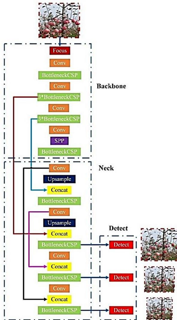
Fig. 3 - The architecture of the original YOLOv5s network
