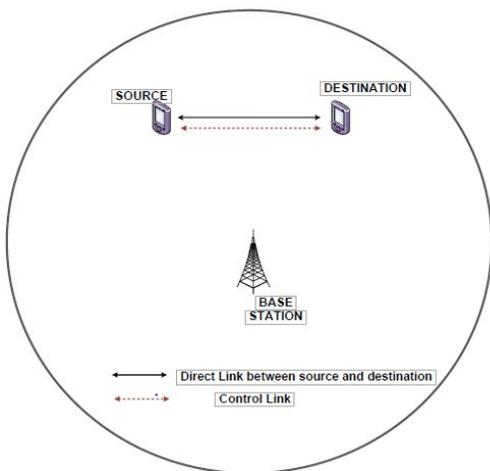
Fig.2. Direct communication between devices (Direct D2D) with device-controlled link establishment.
