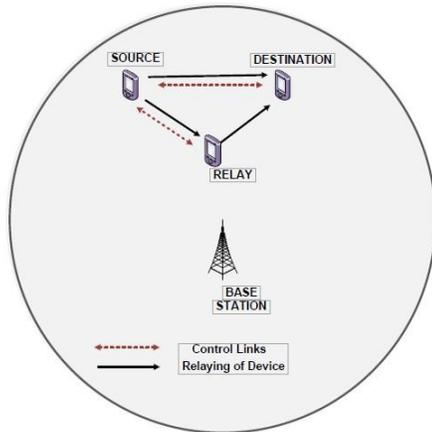
Fig.1. Relaying device with device-controlled link establishment
