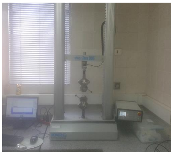
Figure 6. Team KARG industrietechnik model smar Tens 005, equipment used for tensile strength and bending tests.
