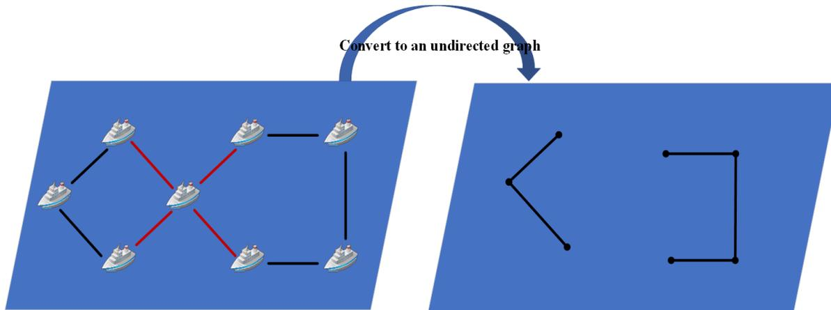
**Figure 6.** The mapping relationship between the formation and the undirected graph when the unmanned ship swarm fails in the unmanned ship swarm.
