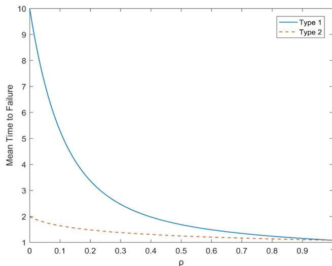
**Figure 5.** For the component types, MTTF vs.  $\rho$ .
