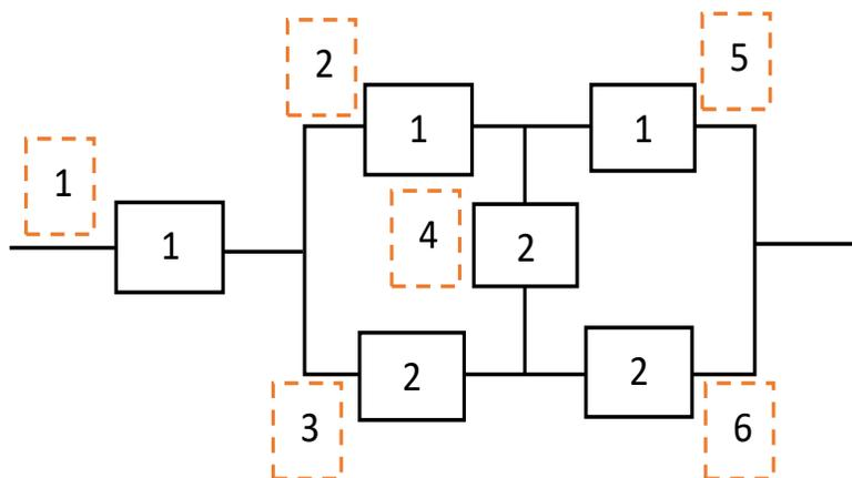
Figure 1. The bridge system with two types of components.
