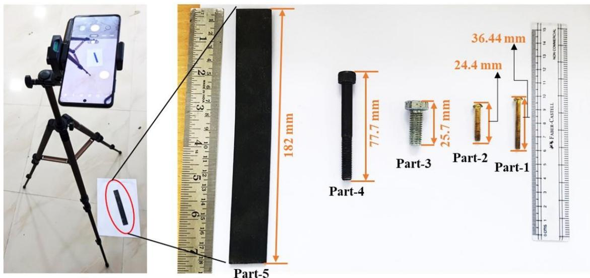
**Figure 1.** Experimental set-up: a) Smartphone camera mounted on tripod stand at a height of 106 cm from ground level and capturing the part-5 (object); b) Various parts/specimens used to validate the proposed technique.
