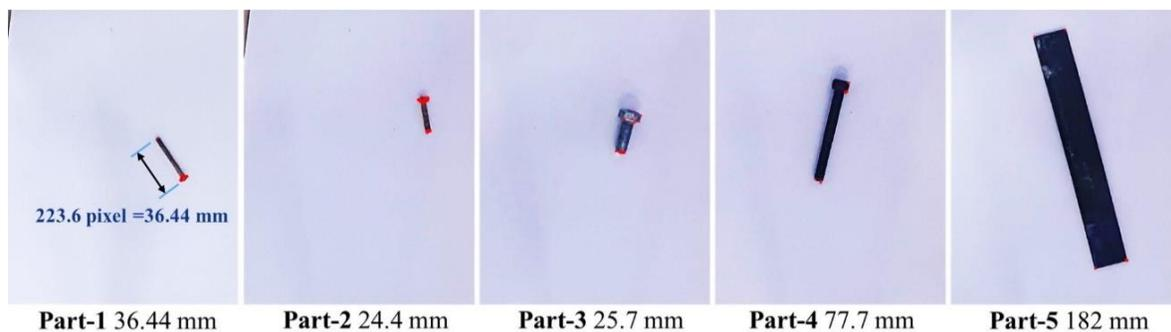
**Figure 2.** Representation of detected corner points (red dot marked) using CV technique for different parts.
