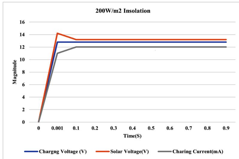
**Figure 11.** Lab performance of solar charger using soft computing technique under 200W/m<sup>2</sup> insolation.
