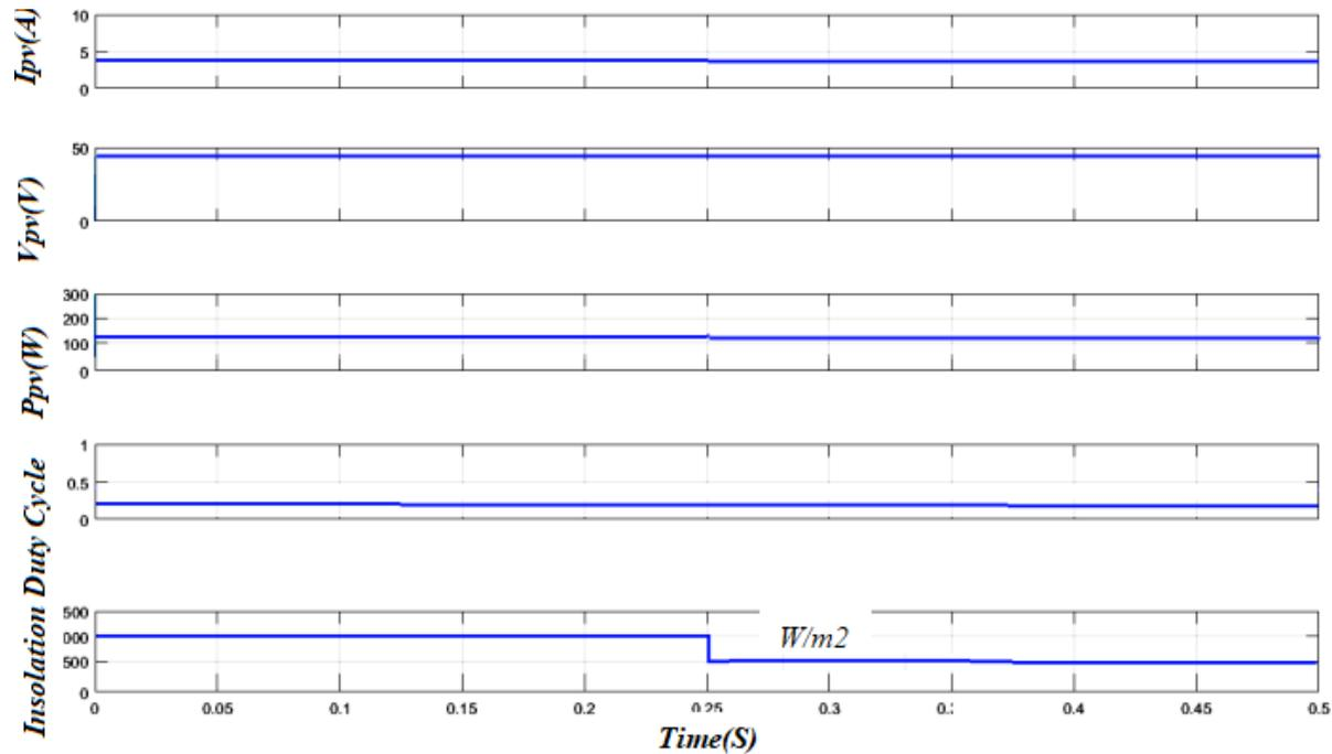
Figure 7. Soft computing based intelligent algorithm performance under 1000w/m2 and 500w/m2 insolation.
