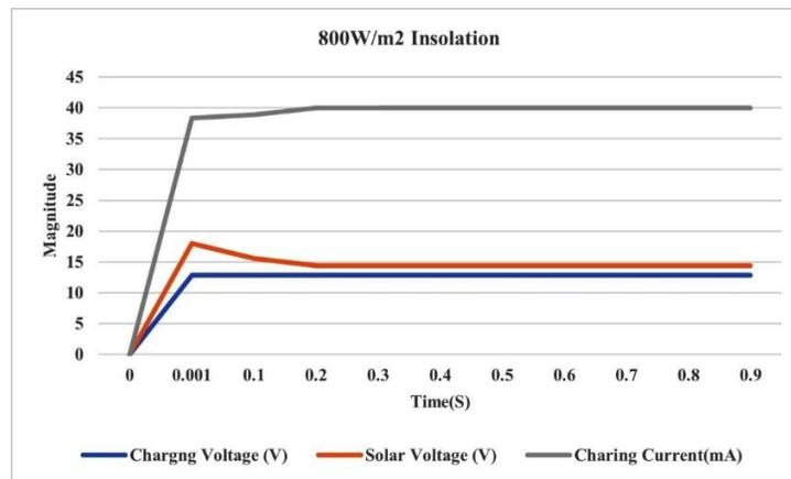
**Figure 9.** Lab performance of solar charger using soft computing technique under 800W/m<sup>2</sup> insolation.
