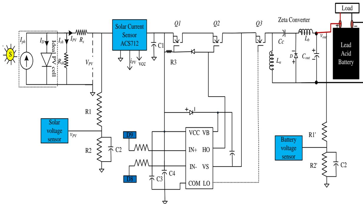
Figure 1. A hardware model of solar battery charger.
