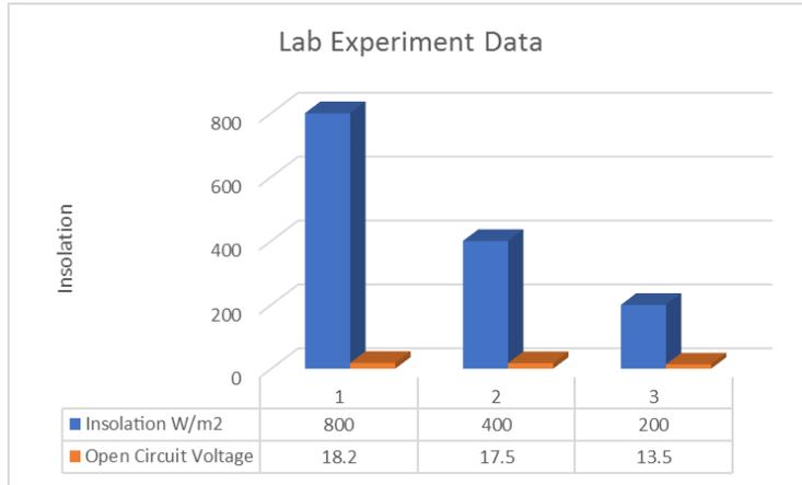
**Figure 8.** Solar panel open circuit voltage under various conditions of insolation.
