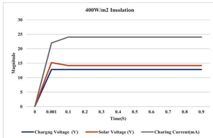
**Figure 10.** Lab performance of solar charger using soft computing technique under 400W/m<sup>2</sup> insolation.
