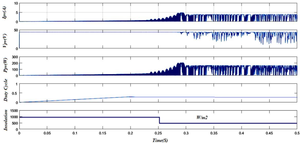
Figure 6. An incremental conductance based algorithm performance under 1000w/m<sup>2</sup> and 500w/m<sup>2</sup> of insolation.
