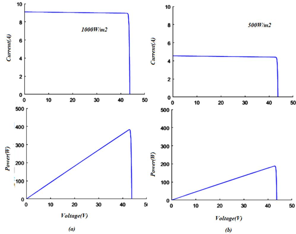
Figure 5 (a)-(b). Characteristics of PV cell under full and partially insolation.
