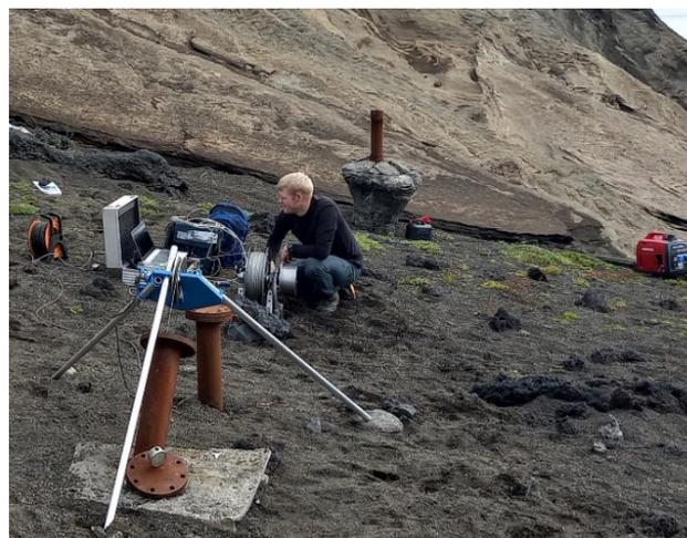
**Figure 2.** Photograph showing ÍSOR logging engineer conducting inclination measurements of the inclined borehole (SE-03) on August 5<sup>th</sup>, 2021.
