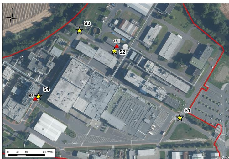
Figure 2: Location of possible ammonia leakage inside of the Seveso establishment
