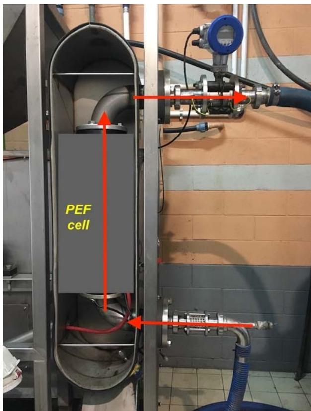
Figure 2: Details of the pulsed electric field (PEF) cell and flow direction
