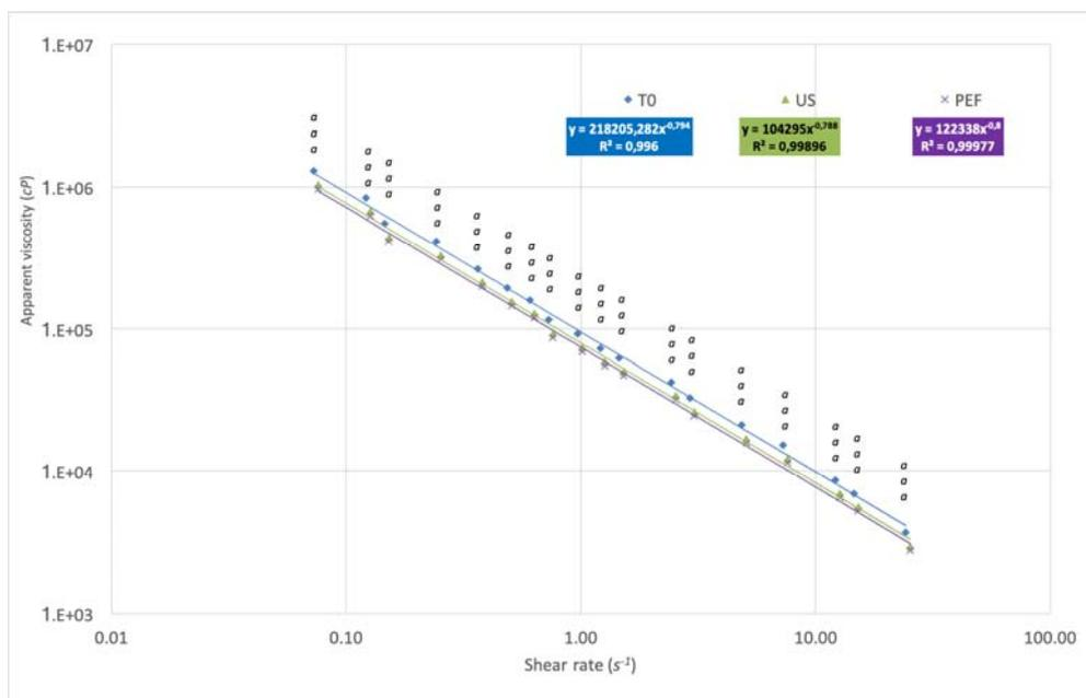
Figure 3: Effect of shear rate on apparent viscosity, plotted in log–log scale, for the two trials (US and PEF), as compared with non-treated olive paste. Different letters denote significant differences (analysis of variance (ANOVA) and honestly significant difference (HSD) test,  $p < 0.05$ ).
