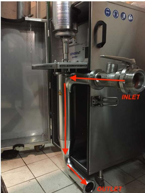
Figure 1: Ultrasound (US) machine, detail of cell flow, US probe and flow direction.
