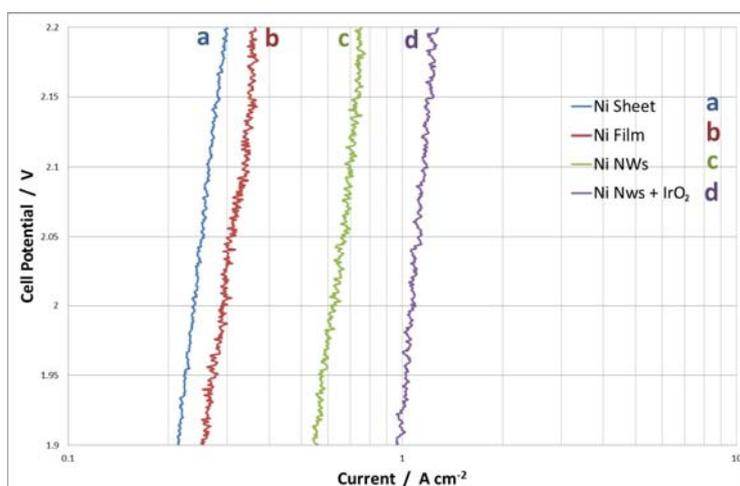
Figure 4 - Quasi-steady-state polarization curves (0.01 V min<sup>-1</sup>) measured for different electrodes in 1 M KOH at room temperature.
