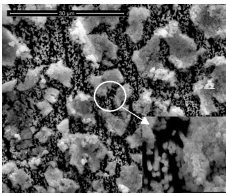
Figure 3 - SEM image, with high magnification inset, of iridium oxide on Ni nanowires after amperostatic deposition at 1 mA cm<sup>-2</sup> for 3 h.
