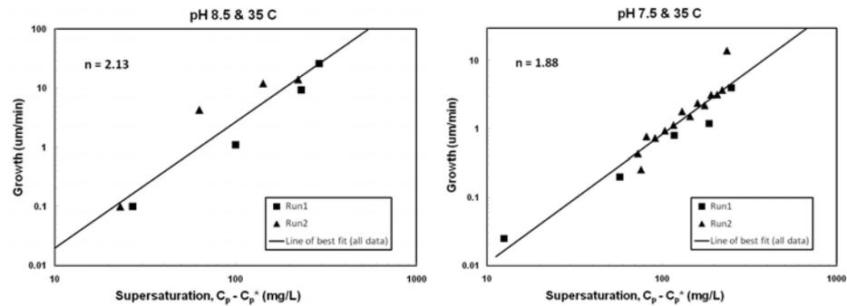
Figure 3: Comparison of growth rates at various supersaturations between duplicate experiments conducted for two conditions at 35 °C, pH 8.5 and pH 7.5.
