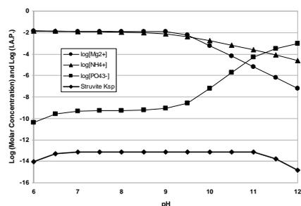
Figure 1: Effect of pH on ionic concentrations when solids are allowed to crystallise, calculated using MINTEQA2. Ionic strength was fixed at 0.1M at 25 °C.
