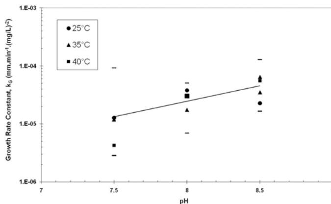
Figure 5: Second order growth rate constant as a function of pH. The line of best fit with pH is shown. The horizontal bars represent the lowest and highest 95 % confidence intervals of  $k_G$  at each pH.
