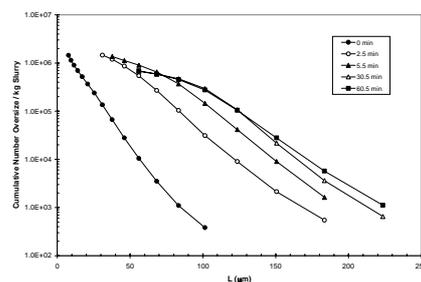
Figure 2: Cumulative number size distributions for the seeded batch crystallisation experiment performed at pH 8.5 and 35 °C.
