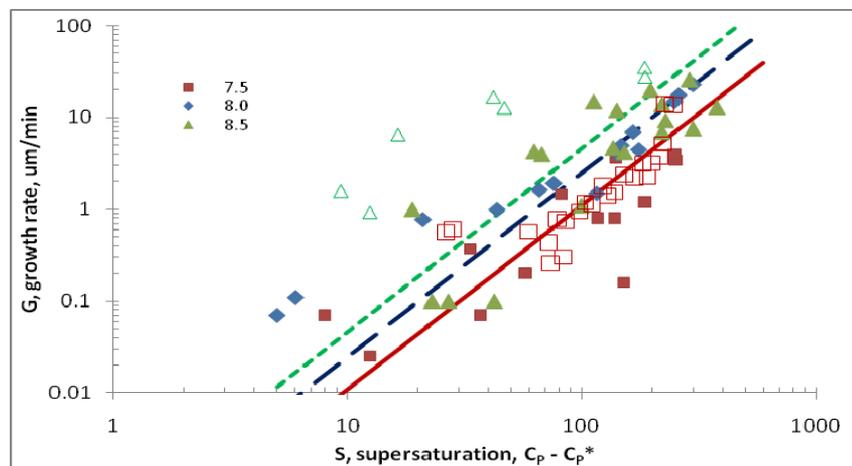
Figure 4: Growth rate versus supersaturation for all experiments. Filled symbols are 1999 data, hollow symbols 2010. Solid line, pH = 7.5, dashed, 8.0, dotted 8.5.
