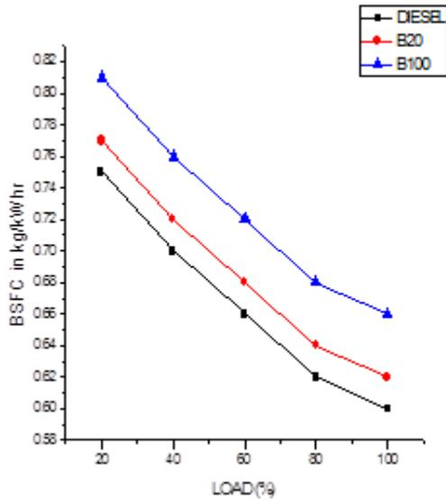
**Fig 5.2 :** Variation in Brake Specific Energy Consumption with Varying Load for Diesel, B20, B100 blends.
