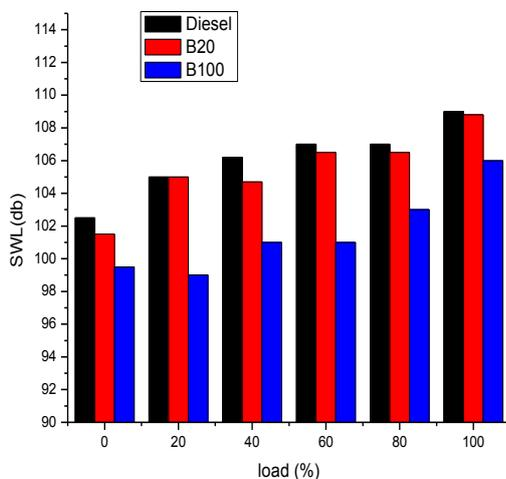
**Fig 5.6:** Variation in Sound Power Level with Varying Load for Diesel, B20& B100 blends
