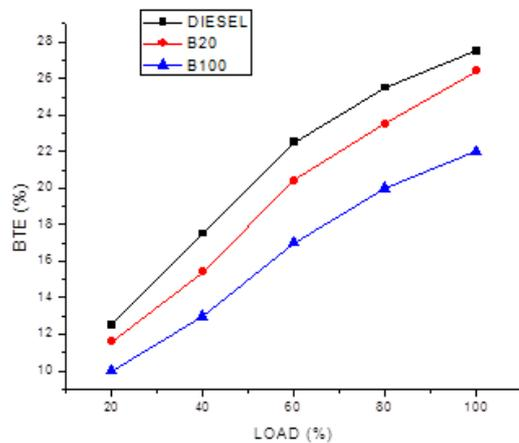
**Fig 5.4 :** Variation in Brake Thermal Efficiency with Varying Load for Diesel, B20 & B100 blends
