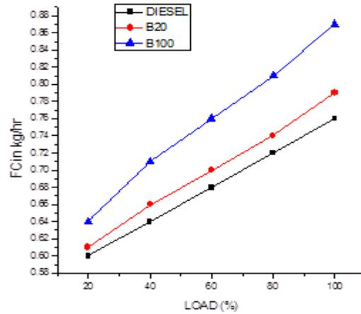
Fig 5.1. Variation in Fuel Consumption with Varying Load for Diesel, B20 & B100 blends
