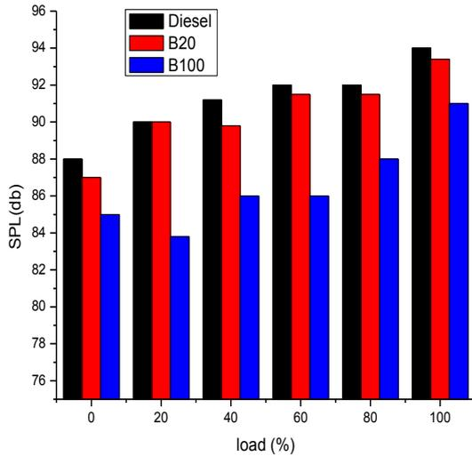
**Fig 5.5 :** Variation in Sound Pressure level with Varying Load for Diesel, B20& B100 blends
