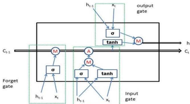
Figure 1 : A typical LSTM repeating memory module structure
