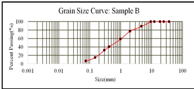
**Figure 3:** Mean particle size distribution curve for Samples from the Farmington Formation
