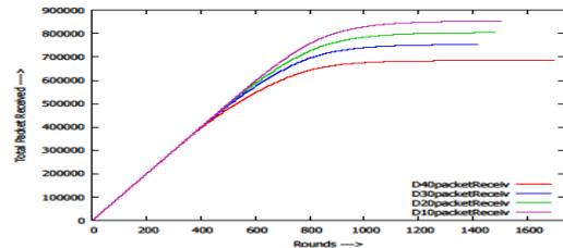
Fig.4.5 : Shows Total packet received by BS in EBBCP for Different value of D
