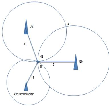
**Fig. 3.2 :** Position finding by Trilateration
