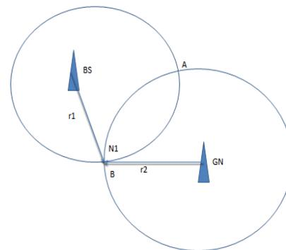
**Fig. 3.1 : Position finding by BS and GN (Lateration)**
