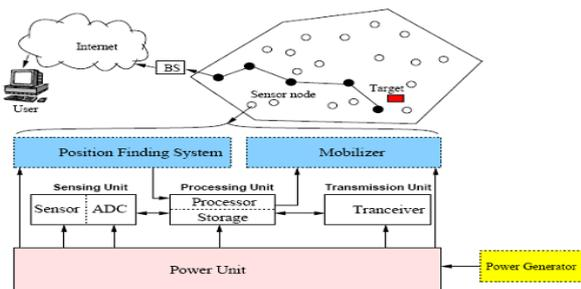
Fig.2.2 : Sensor node architecture
