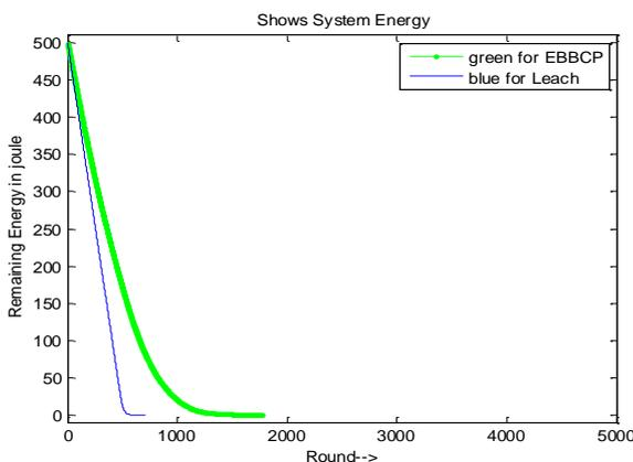
**Fig.4.7 :** Comparison of Network Remaining Energy in EBBCP and LEACH
