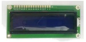
LCD screen is used for showing the status of the process being run on the device. The screen is usually monochrome and connects to the Arduino via special connector.
