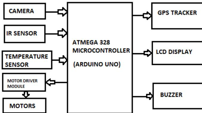
Fig 1: Block Diagram Of Underground Cable Connection Fault Detecting Robot
