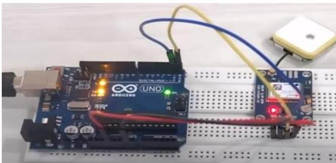
Fig3: Connecting GPS Tracker with Arduino
