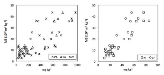
Figure 2. Relationships between trace element contents and magnetic susceptibility (MS) in the compost size fractions.
