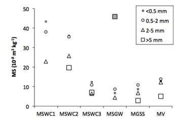
Figure I. Magnetic susceptibility (MS) of the composts' size fractions.
