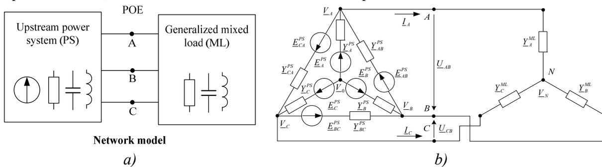
Fig. 1. The equivalent circuit of a power supply system with separately presented POE nodes in phase coordinates: a) common diagram, b) detailed model with configurations of the upstream power system and generalized mixed load equivalent circuits
