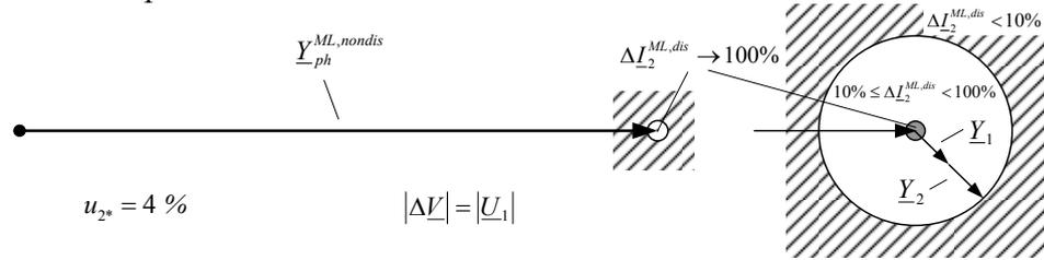
Fig. 4. Relative error for the identification of a voltage unbalance emission source
