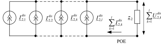
Fig. 3. The equivalent circuit of a power supply system for the negative sequence components
