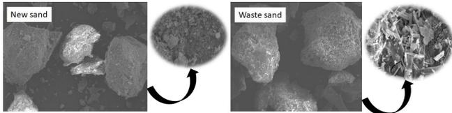
**Figure 5:** The morphology of new sand and waste sand
