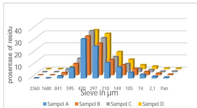
**Figure 4:** Distribution size of A) waste sand without washing, B) detergent whased 0.2%, C) detergent whased 0.3%, dan D) detergent whased 0.4%
