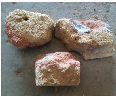
**Figure 1:** The lump of CO<sub>2</sub> waste moulding sands
