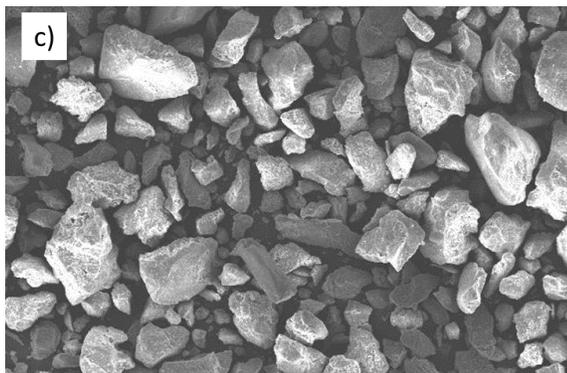
**Figure 2:**The grain shapes of a) new sand, b) sand waste without washing, dan c) sand waste with washing
