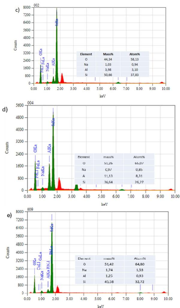
**Figure 7:** Element content of a) new sand, b) waste sand without washing, c) detergent washed 0.2%, d) detergent washed 0.3%, e) detergent washed 0.4%
