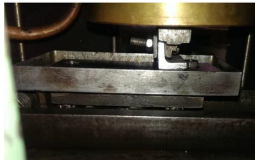
Figure 8: Sample in holder for wear tests.
