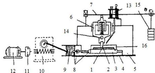
**Figure 6:** 77 MT-1 friction testing machine: 1 –cylinder sample; 2 – piston ring sample; 3 –crosshead; 4 – guide; 5 – machine body; 6 – rod; 7 – load lever; 8 – pivots; 9 –sliding block; 10 – reducer; 11 – coupling; 12 – electromotor; 13 – oiler; 14 –heater; 15 – weight; 16 – oiling tank.
