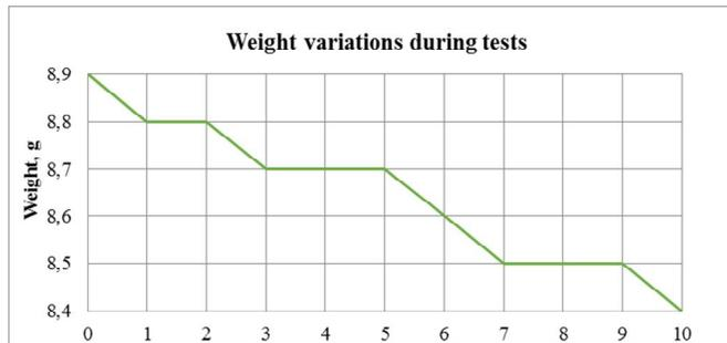
**Figure 10:** Weight loss of sample coated with Ceramic T in 10 h.
