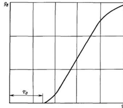
**Figure 4:** Weight loss of tested sample as a function of wear duration.
