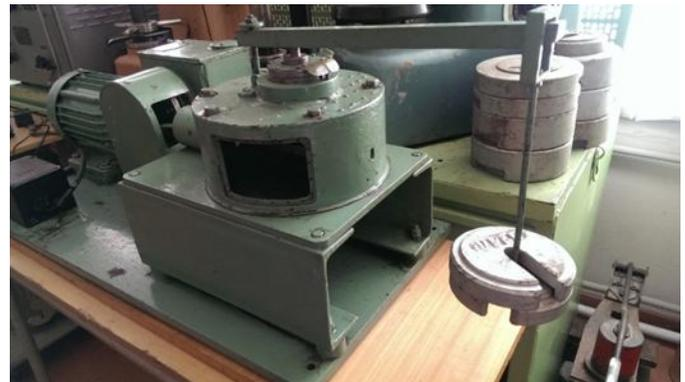
**Figure 5:** 77 MT-1 friction testing machine.
