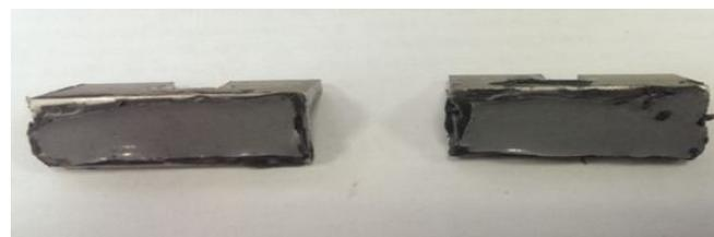
**Figure 2:** Sample (angle) with applied material for wearing tests
