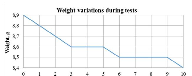
Figure 9: Weight loss of sample coated with Ceramic F in 10 h.
