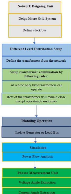
**Figure 1:**Methodology to determine voltage angle and current angle of the islanding event
