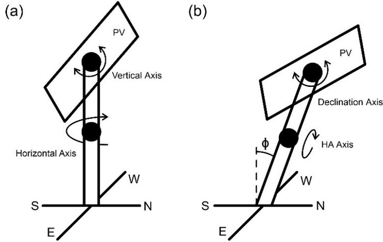
FIGURE 3. Types of dual-axis solar tracker: (a) Polar and (b) azimuthal
