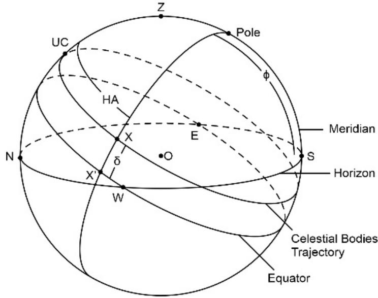
FIGURE 1. Celestial bodies (X) position on equatorial mount system
