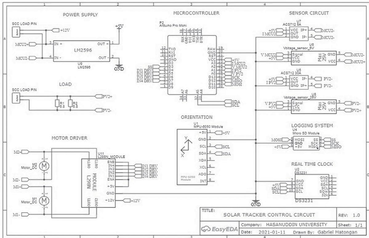
FIGURE 5. Wiring diagram of electrical and control components
