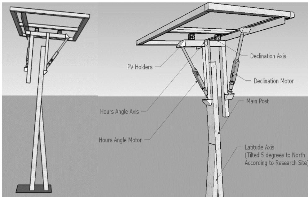
FIGURE 4. Mechanical structure of polar dual-axis solar tracker
