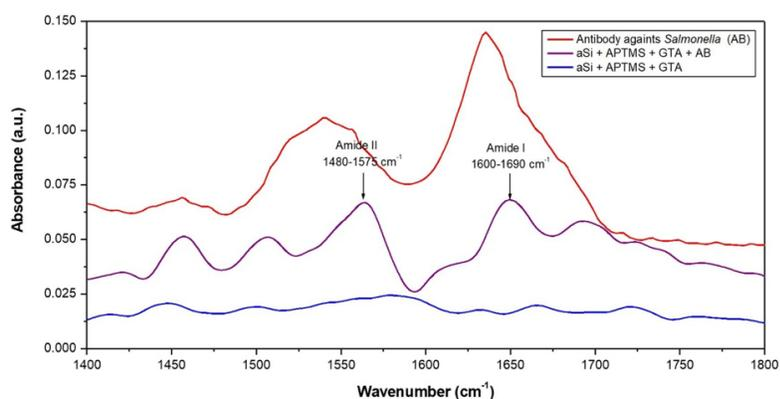
Fig. 7. Biofunctionalization IR spectra on amorphous silicon substrates, analyzed in transmission mode.
