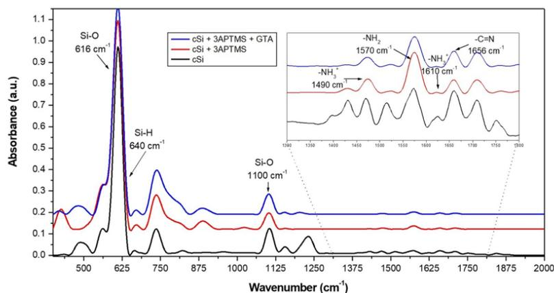
Fig. 5. IR spectra of GTA functionalization on crystalline silicon substrates, analyzed in transmission mode.
