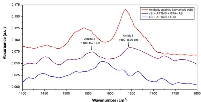
Fig. 8. Biofunctionalization IR spectra on crystalline silicon substrates, analyzed in transmission mode.
