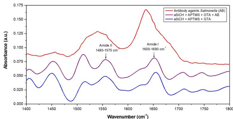
Fig. 9. Biofunctionalization IR spectra on hydrogenated amorphous silicon carbide substrates, analyzed in transmission mode.
