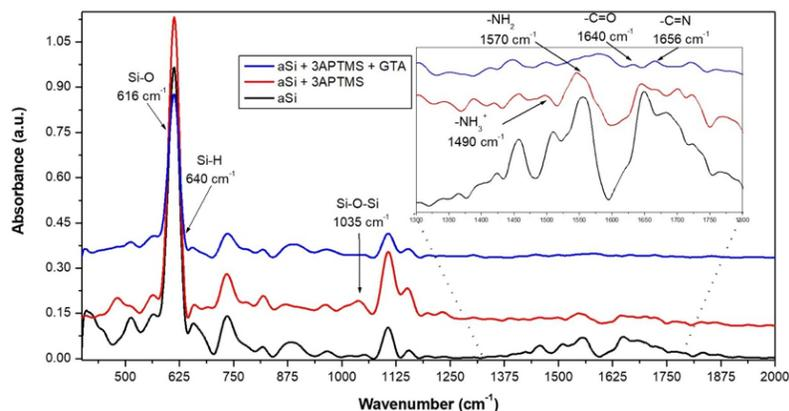
Fig. 4. IR spectra of GTA functionalization on amorphous silicon substrates, analyzed in transmission mode.
