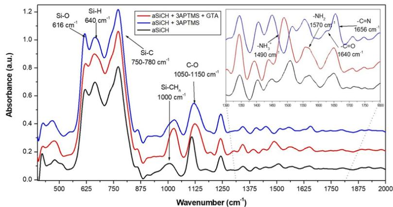
Fig. 6. IR spectra of GTA functionalization on hydrogenated amorphous silicon carbide substrates, analyzed in transmission mode.
