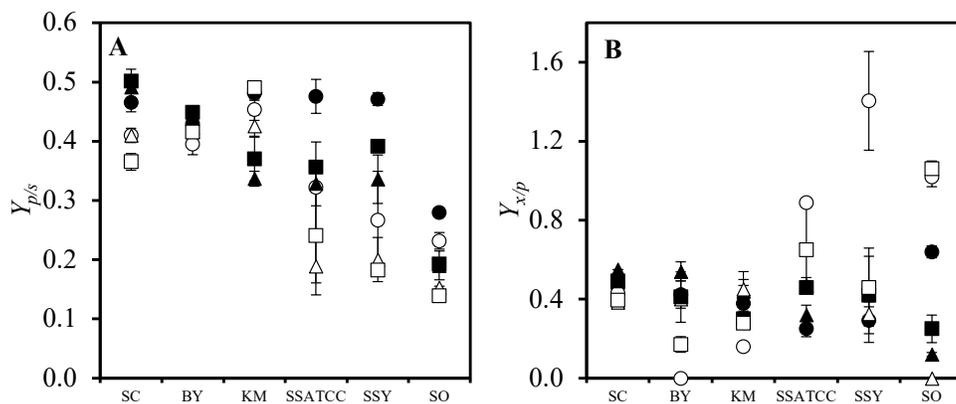
Figure 4. A)  $Y_{p/s}$  and B)  $Y_{x/p}$  obtained during the yeast assays in the three flask designs: conventional (●, ○), coiled (▲, △), and baffled (■, □). Filled and empty symbols correspond to a filling volume of 20 and 40 %, respectively. *S. cerevisiae* ITD00196 (SC); baker's yeast (BY); *K. marxianus* CBS6556 (KM); *S. stipitis* ATCC58785 (SSATCC); *S. stipitis* Y-17104 (SSY); *Schw. occidentalis* ATCC26077 (SO).
