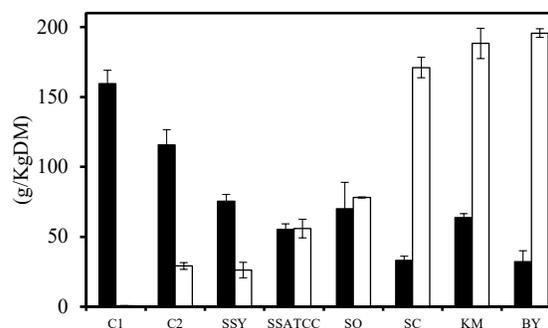
Figure 5. Ethanol (open bars) and fermentable carbohydrates (filled bars) using different yeasts in the fermentation of the SSM without pre-treatment. Control 1 (C1) at the initial time, Control 2 (C2) at the final time (30 h). *S. cerevisiae* ITD00196 (SC); baker's yeast (BY); *K. marxianus* CBS6556 (KM); *S. stipitis* ATCC58785 (SSATCC); *S. stipitis* Y-17104 (SSY); *Schw. occidentalis* ATCC26077 (SO).
