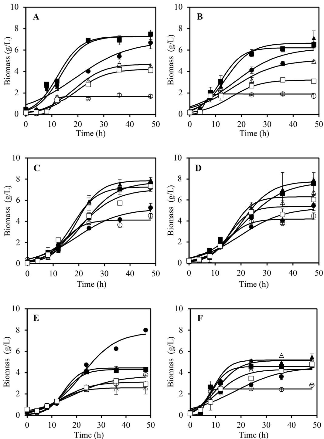
Figure 1. Growth curves in the three flask designs: conventional (●, ○), coiled (▲, △) and baffled (■, □). Filled and empty symbols correspond to a filling volume of 20 and 40 %, respectively. The continuous line corresponds to the fit of the integral logistic model to the growth curves of the yeasts: A) *S. cerevisiae* ITD00196; B) baker's yeast; C) *S. stipitis* ATCC58785; D) *S. stipitis* Y-17104; E) *Schw. occidentalis* ATCC26077; F) *K. marxianus* CBS6556.
