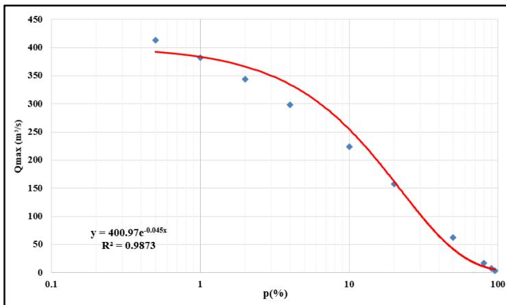
**Fig. 7.** The theoretical distribution curve Log Pearson III of the maximum annual discharges of Cotmeana River at Ciobani (1964-2014)
