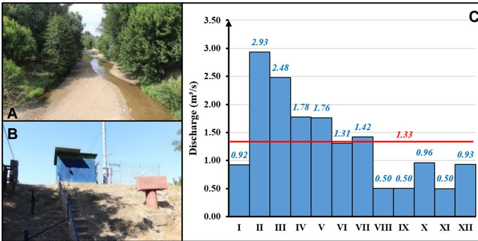
**Fig. 2.** The Cotmeana river characteristics. A) Cotmeana river; B) Ciobani gauging station; C) Monthly mean discharges (1964-2014)
