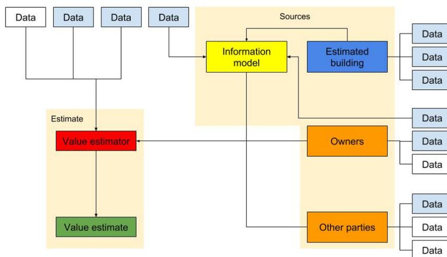
Fig. 2. Simple BIM approach (Level 2) schematics
