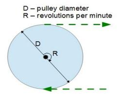
Belt Speed (BS): The calculator computes the belt speed in feet per second. However, this can be automatically converted to other velocity units via the pull-down menu.
