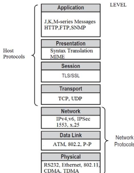
**.Figure 3. The equivalent ISO OSI reference model [1]**
