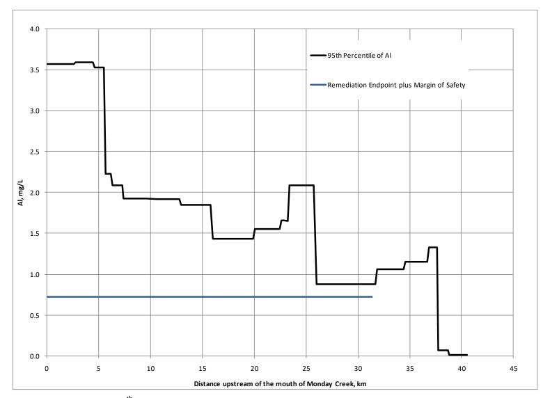
Figure 7. Plot of the 95<sup>th</sup> percentile of the simulated aluminum for the Monday Creek main stem after the activation of the Jobs Hollow doser.
