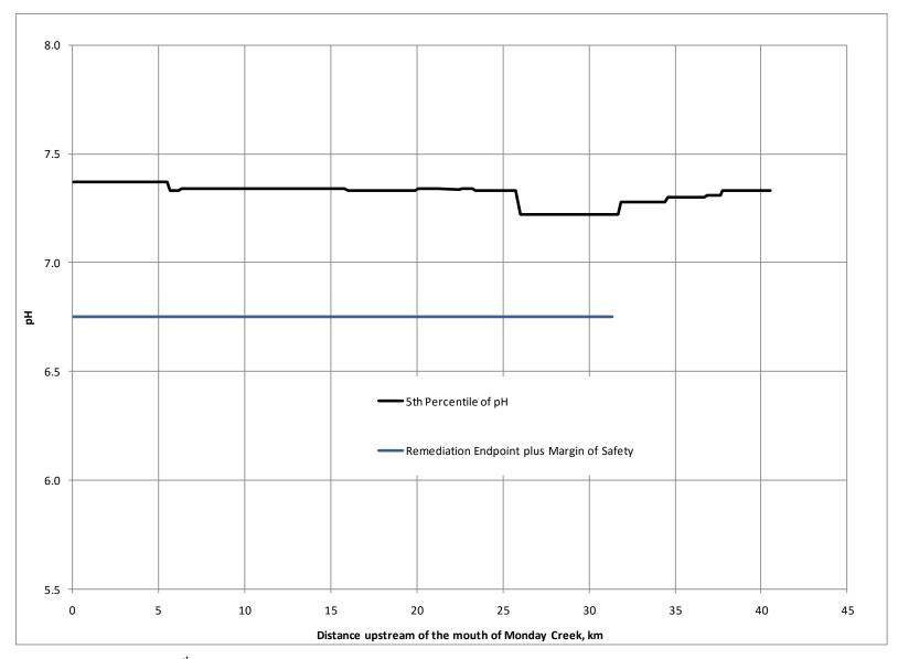
Figure 10. Plot of the 5<sup>th</sup> percentile of the simulated main stem pH with Treatment Alternative 1.
