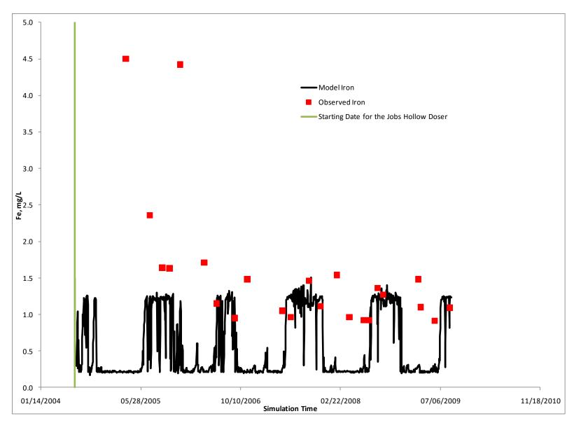
Figure 5. Simulated and observed iron at MC-127 from the calibrated Monday Creek model.
