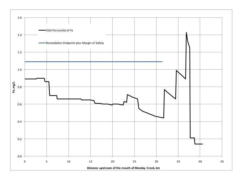
Figure 8. Plot of the 95<sup>th</sup> percentile of the simulated iron for the Monday Creek main stem after the activation of the Jobs Hollow doser.
