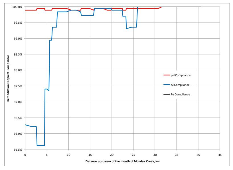
Figure 17. Compliance plot for the simulated pH, aluminum, and iron with Treatment Alternative 2.
