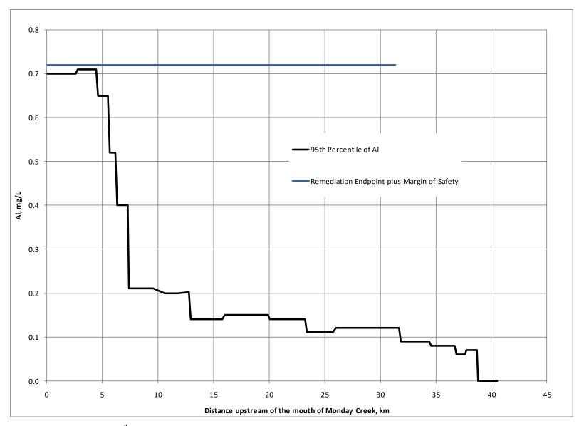
Figure 15. Plot of the 95<sup>th</sup> percentile of the simulated main stem aluminum with Treatment Alternative 2.
