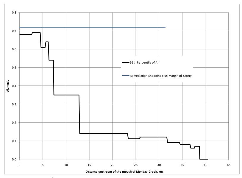
Figure 11. Plot of the 95<sup>th</sup> percentile of the simulated main stem aluminum with Treatment Alternative 1.
