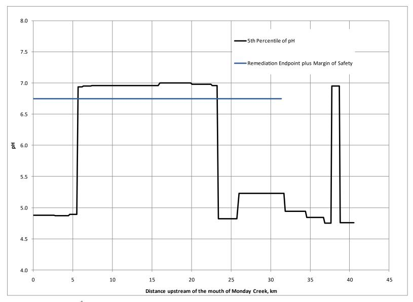
Figure 6. Plot of the 5<sup>th</sup> percentile of simulated pH for the Monday Creek main stem after the activation of the Jobs Hollow doser.
