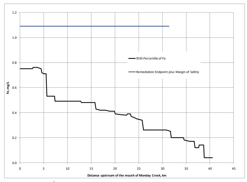
Figure 16. Plot of the 95<sup>th</sup> percentile of the simulated main stem iron with Treatment Alternative 2.
