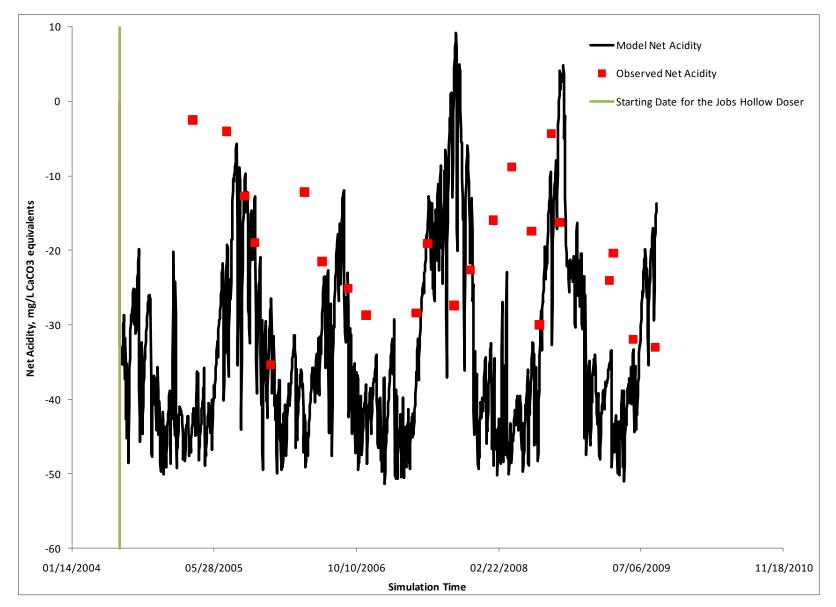
Figure 2. Simulated and observed net acidity at MC-127 from the calibrated Monday Creek model.
