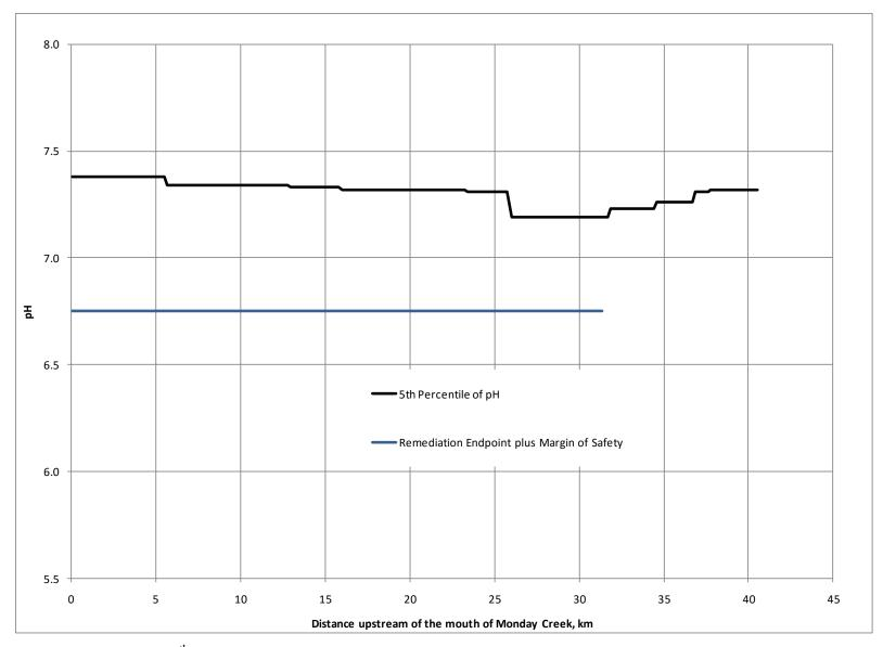
Figure 14. Plot of the 5<sup>th</sup> percentile of the simulated main stem pH with Treatment Alternative 2.
