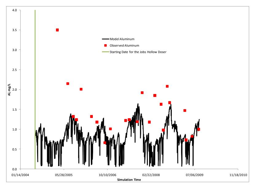
Figure 4. Simulated and observed aluminum at MC-127 from the calibrated Monday Creek model.
