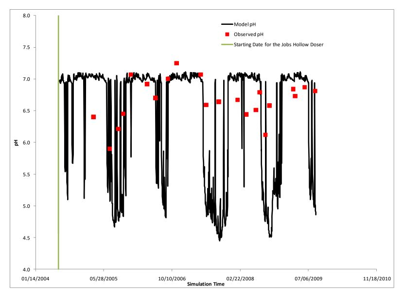
Figure 3. Simulated and observed pH at MC-127 from the calibrated Monday Creek model.
