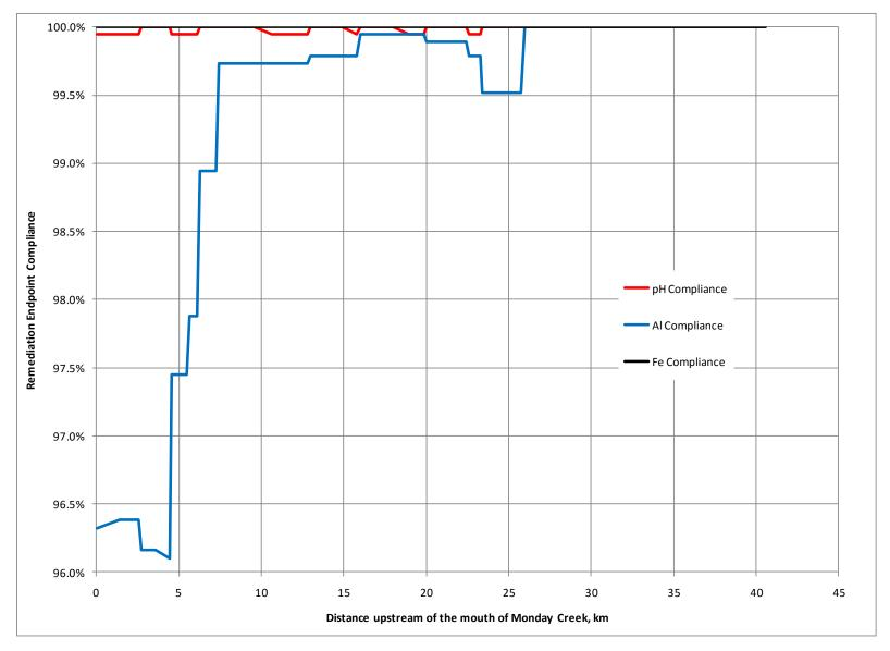
Figure 13. Compliance plot for the simulated pH, aluminum, and iron with Treatment Alternative 1.
