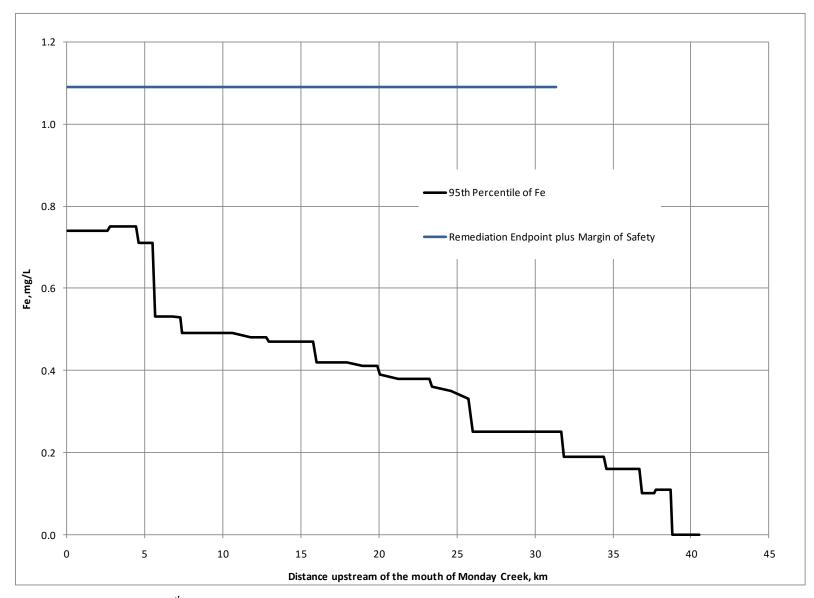
Figure 12. Plot of the 95<sup>th</sup> percentile of the simulated main stem iron with Treatment Alternative 1.
