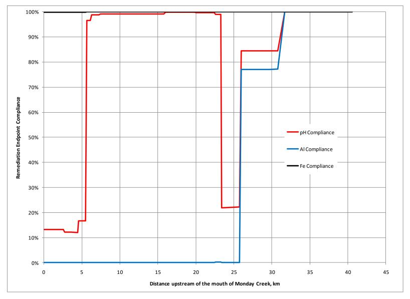
Figure 9. Plot of the compliance of the simulated pH, aluminum, and iron from the calibration model with the remediation endpoints.
