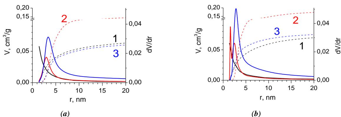
**Figure 3. Integral and differential pore size distributions calculated from BJH theory using the adsorption (a) and desorption (b) branches of isotherms for MS-1 (1), K1 (2), and K2 (3).**
