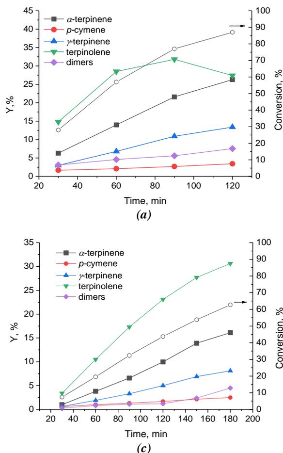
**Figure 7.** Conversion, product yields (a, c) vs. reaction time, and selectivity vs. conversion (b, d) on the samples K2 (a, b) and K1 (c, d).
