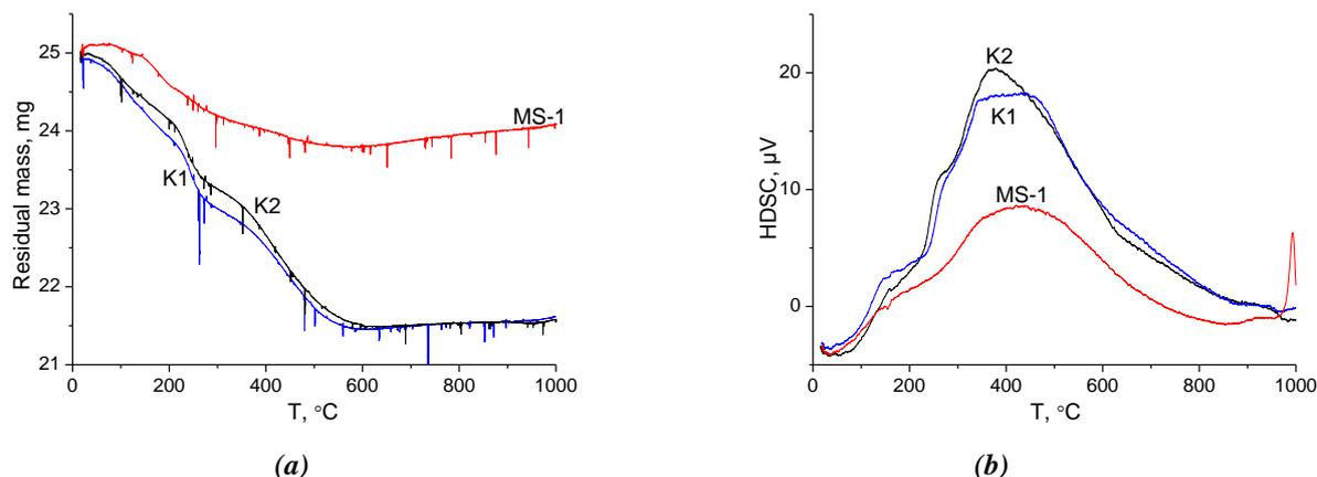
**Figure 8.** TG (a) and DTA (b) curves of MS-1, K1, and K2 deactivated samples.
