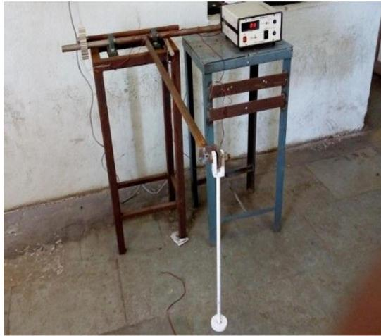
Figure 5 Loading arrangement of gear pair
