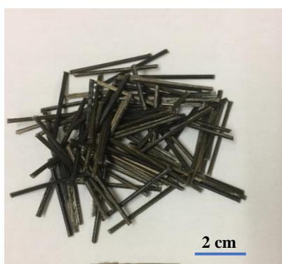
Figure 1-Reinforcing basalt fiber pellets.
