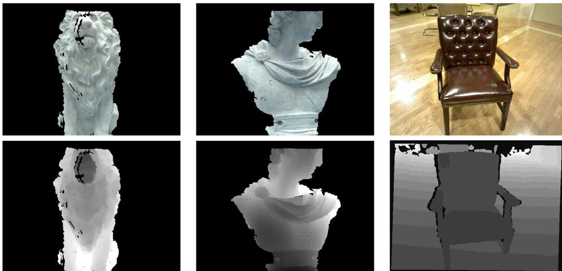
**Figure 1.** RGB images and depth maps of a lion, an apollo, and a chair are scanned by Kinect sensor.
