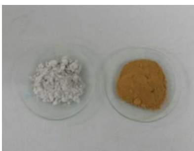
Figure 2. LGL before and after reaction with AMD sample
