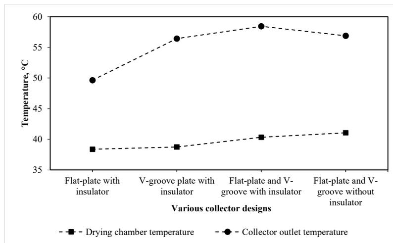
FIGURE 5. The drying chamber and collector outlet temperature against various collector designs
