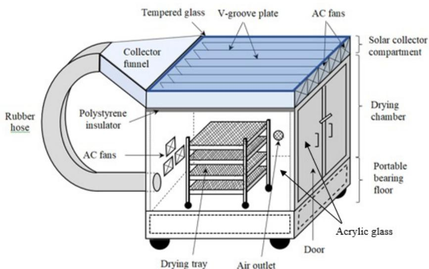
FIGURE 1. Schematic of the portable solar greenhouse dryer
