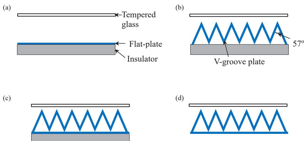
FIGURE 2. The solar collector arrangement of (a) flat-plate with insulator, (b) V-groove with insulator, (c) flat-plate and V-groove with insulator and (d) flat-plate and V-groove without insulator
