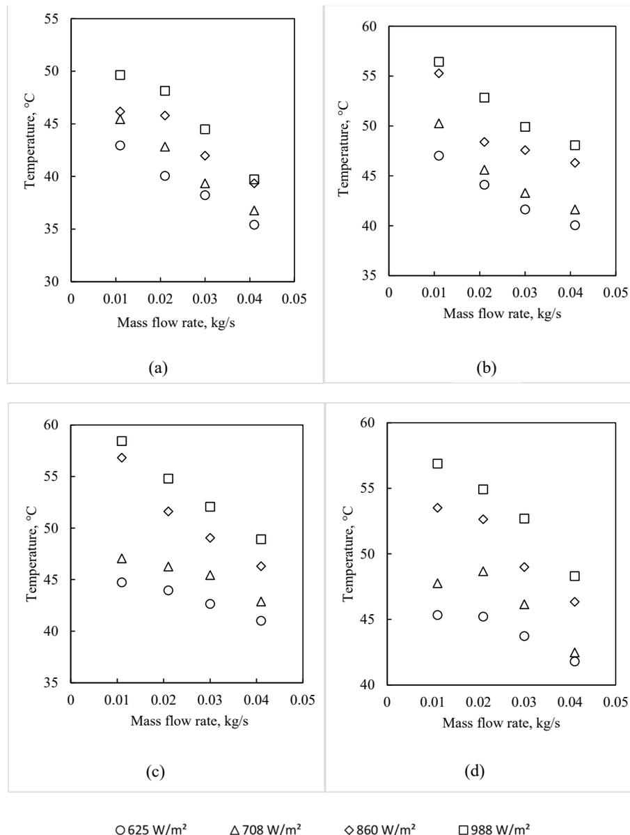
FIGURE 3. The collector outlet temperature with mass flow rate at different solar radiation for (a) flat-plate with insulator, (b) V-groove with insulator, (c) Flat-plate and V-groove with insulator and (d) flat-plate and V-groove without insulator
