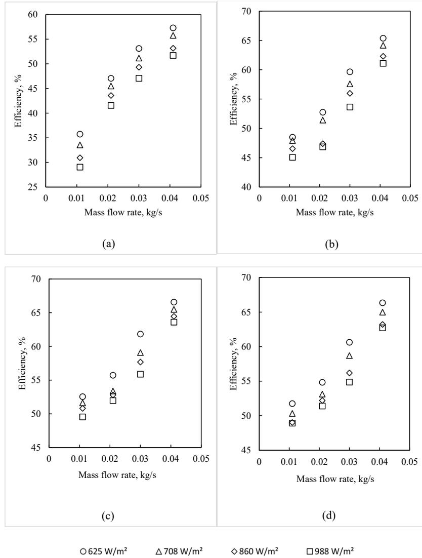
FIGURE 4. The efficiency change with mass flow rate at different solar radiation for (a) flat-plate with insulator, (b) V-groove with insulator, (c) Flat-plate and V-groove with insulator and (d) flat-plate and V-groove without insulator
