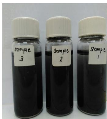
FIGURE 1. Graphene suspensions from samples prepared at different ball milling speeds for 30 min. (1) at speed 100 rpm, and (2) at 500 rpm. Pictures taken for composite samples dispersed in DW after 1 h sonication
