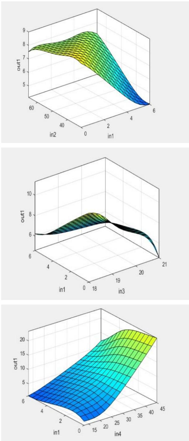
FIGURE 5. Parametric study of the variables' effects on swell potential of the treated expansive soil from ANFIS model
