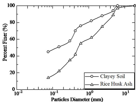
FIGURE 1. Particle size distribution curve of the clayey soil and rice husk ash
