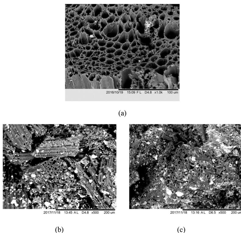
FIGURE 3. The morphology of activated carbon: (a) before adsorption; (b) after adsorption for 50 mg/L of Hg(II) initial concentration, 20 mL/min of flow rate of; and (c) after adsorption for 100 mg/L of Hg(II) initial concentration, 20 mL/min of flow rate
