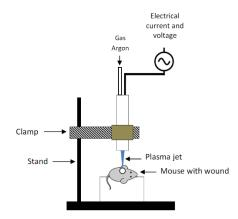
Figure 1: Plasma treatment experimental set-up
