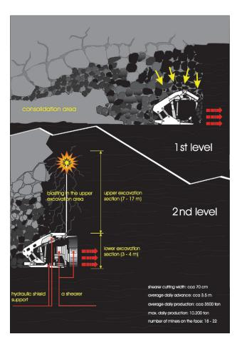
**Figure 3:** Cross-section of the hydraulic shield support with the principle of mining in the Velenje Colliery<sup>4</sup>
