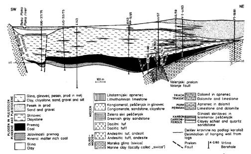
**Figure 2:** Cross-section through the Velenje depression oriented NE-SW, with underground outline of the coal seam<sup>3</sup> **Slika 2:** Presek skozi velenjsko depresijo, orientirano SV-JZ s podzemnim prikazom ležišča premoga<sup>3</sup>
