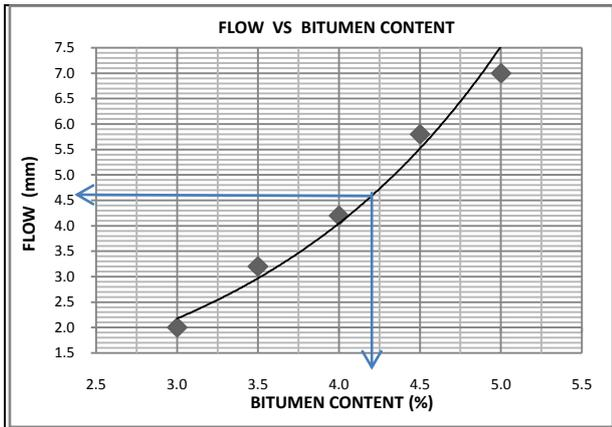
Figure 5:- Flow V/s. Bitumen Content
