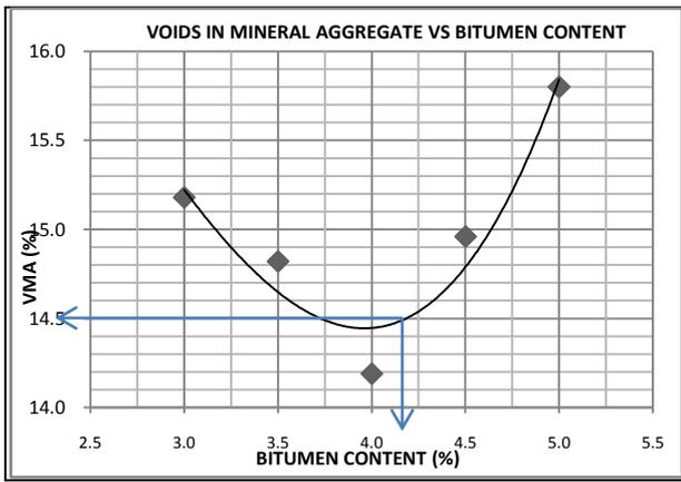
Figure 4:- Voids in Mineral Aggregate V/s. Bitumen Content
