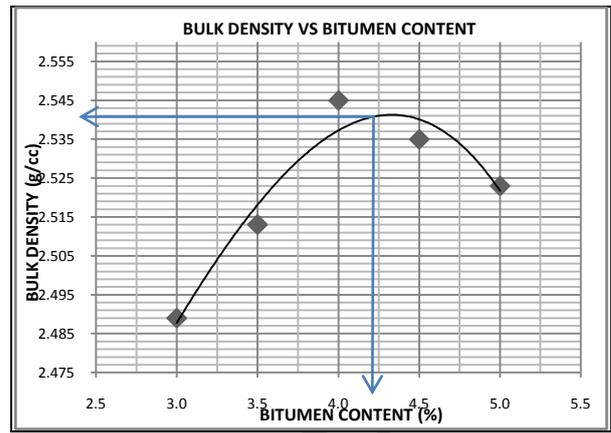
Figure 6:- Bulk Density V/s. Bitumen Content
