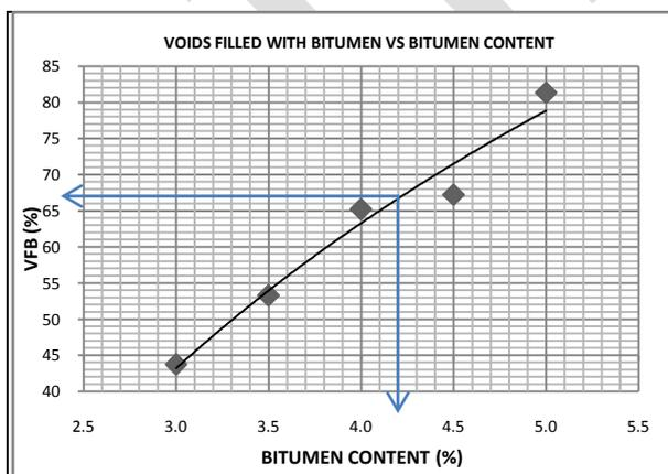
Figure 2:- Voids Filled with Bitumen V/s. Bitumen Content
