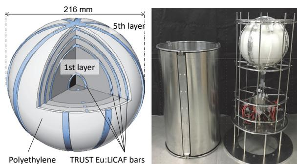
Figure 1. Conceptual drawing and photograph of the fabricated onion-like single Bonner sphere detector.
