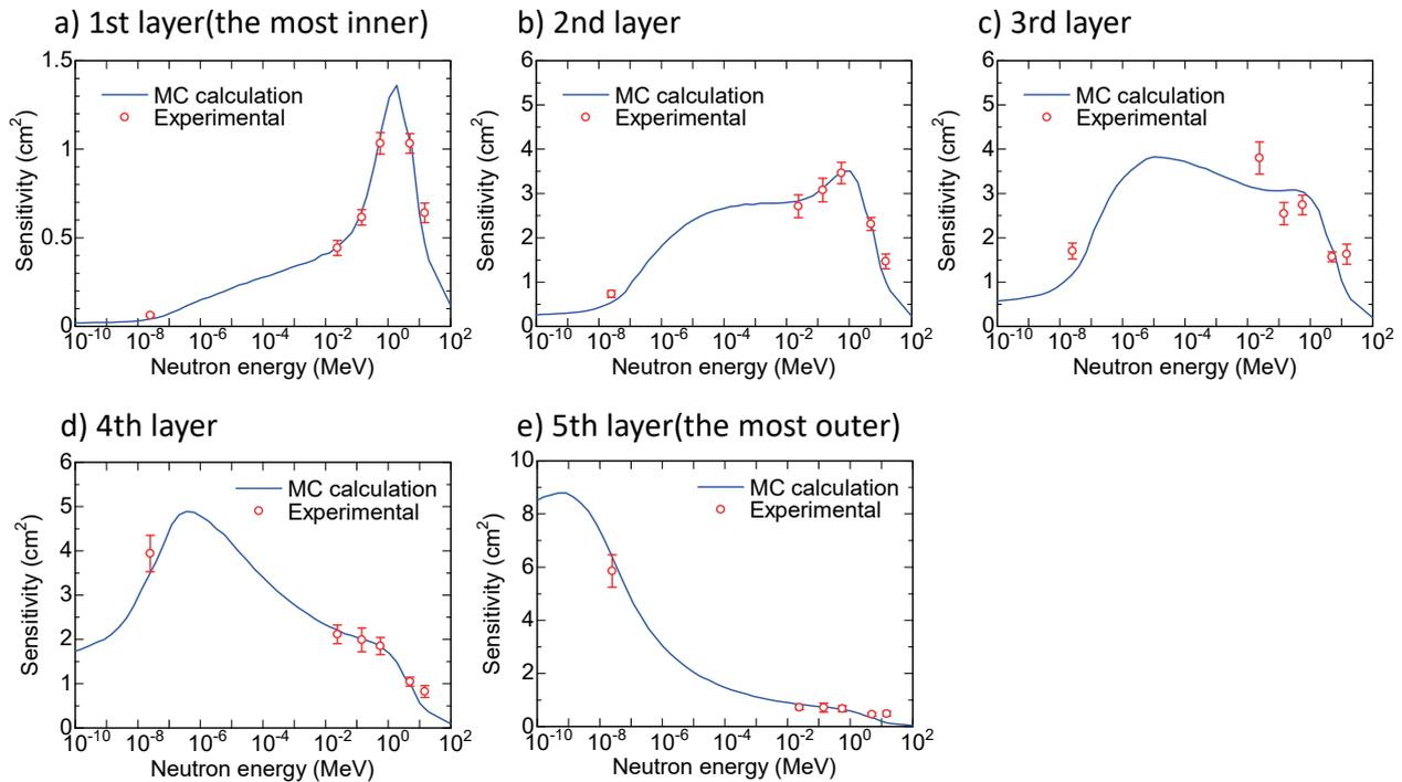
Figure 3. Energy dependence of the experimentally determined detector sensitivities of each sensitive layer (open circles). The Monte Carlo calculation results are also plotted (solid lines). The calculated responses are corrected by taking into account of the counting efficiency.
