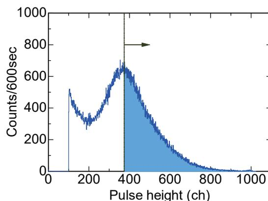
Figure 2. Example of the pulse height spectrum obtained from the fabricated detector. The data were taken from the fourth layer from the most inner shell when irradiating 144 keV neutrons.
