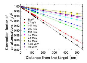
Figure 8. Correction factor of the air attenuation  $F_A(d)$  as a function of the distance from the target. These data were calculated using the MCNP-ANT code.
