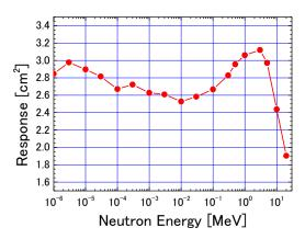
Figure 4. Response of the Long Counter calculated using the MCNP-4C code. The response was determined from the number of  ${}^{10}B(n,\alpha)^7Li$  reaction in the sensitive area of the BF<sub>3</sub> counter. The shape of the response curve for the  ${}^{3}He$  counter is quite similar to that of the BF<sub>3</sub> counter.
