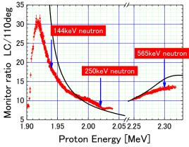
Figure 9. Relationship between proton energy and count ratio of the LC and the 110deg-monitor for  $^{7}Li(p,n)^{7}Be$  reaction.
