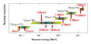
Figure 1. Available energy points and nuclear reactions employed for neutron production in the mono-energetic neutron calibration fields.
