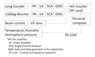
Figure 7. Block diagram of the developed neutron fluence monitoring system.
