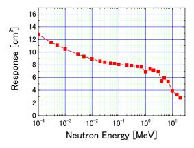
Figure 6. Response of the 110deg-monitor calculated by using the MCNP-4C code. The response was determined from the number of  ${}^{3}$ He(n,p) ${}^{3}$ H reaction in the sensitive area of the  ${}^{3}$ He counter.
