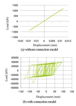
Fig. 19 Load-displacement relation at the joint (Model 1, top of IHX)
