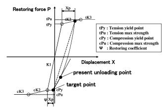
Fig. 5 Hysteresis characteristics of each spring (Ramberg-Osgood model)
