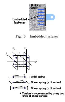
Fig. 4 Spring model of elastic-plastic connection
