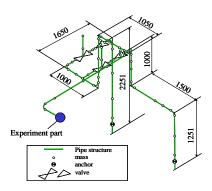
Fig. 13 Whole system including the piping support
