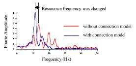
Fig. 21 Comparison of the frequency response at the top of IHX (Model 1, x direction)
