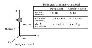
Fig. 14 Analytical model and the parameters
