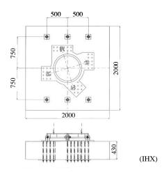
Fig. 9 Equipment support experimental specimen
