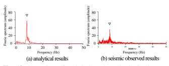
Fig. 18 Comparison of analytical results and seismic observations (Model 1, top of IHX)
