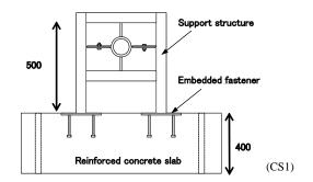
Fig. 8 One kind of piping support experimental specimens
