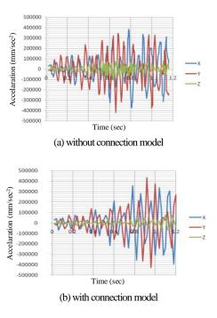
Fig. 20 Comparison of time response at the top of IHX (Model 1)
