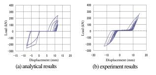
Fig. 16 Load-displacement relation (seismic loading of equipment support)
