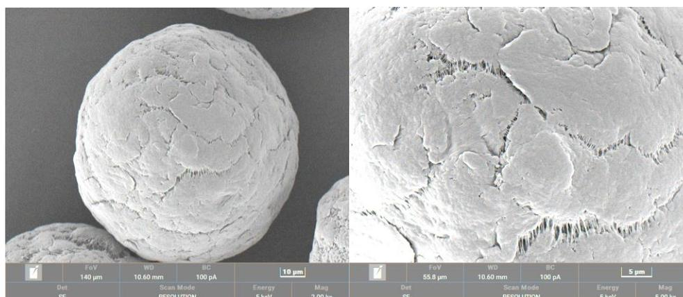
**Figure 1.** SEM of PE
