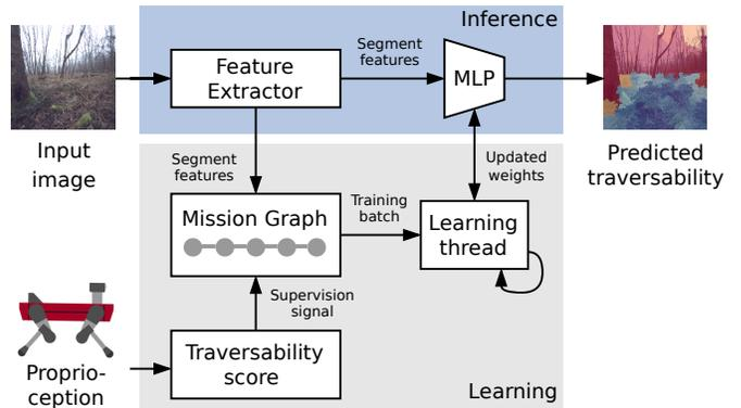
Fig. 2: System overview: **WVN** only requires monocular RGB images and proprioceptive data as input, which are processed to extract features and supervision signals used for online learning and inference of traversability (see Sec. III).
