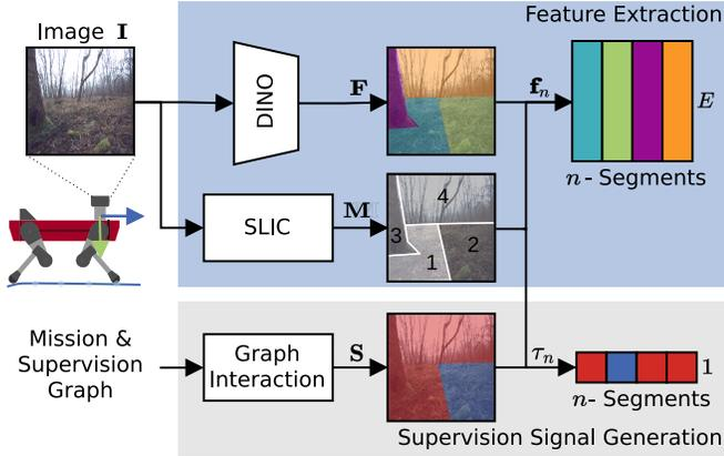
Fig. 3: Feature Extraction: Our approach extracts dense DINO-ViT features  $\mathbf{F}$  from an RGB image  $\mathbf{I}$ , and  $n = 100$  segments  $\mathbf{M}$  using SLIC. For each of the  $n$  segments we average the corresponding features to obtain per-segment embeddings  $\mathbf{f}_n$ . A traversability score  $\tau_n$  is computed for each segment based on the score resulting from the graph interaction process (for more detail refer to Sec. III-D).
